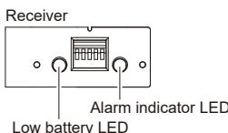
4 Conduct a walk test to check that the alarm indicator LED on the receiver turns ON as the walker interrupts the beams.
