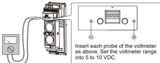
5 Continue the fine alignment until it reaches maximum monitor output over "good" level.
