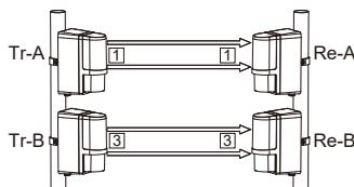
Since Receiver B may receive the infrared beam from Transmitter A, select the frequencies as shown in the figure on the left. (In the figure, each number in the square indicate a channel numbers.)
