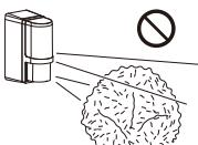
Do not install the receiver in a location where it is exposed to direct sunlight.
