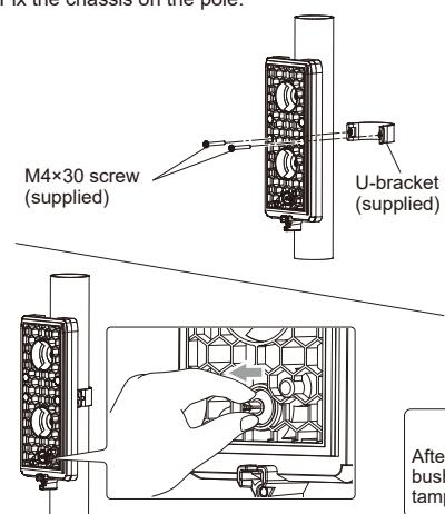
3 Install three pole mounting brackets on the chassis.
