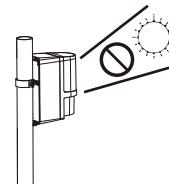
Do not allow the infrared beam from a different model to reach the receiver.
