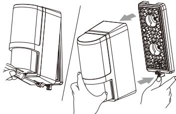
2 Fix the chassis to the wall.
