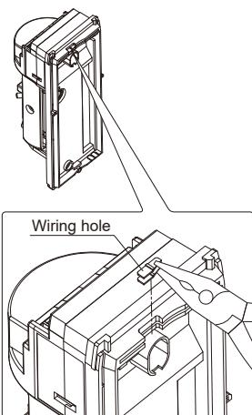
5 Remove the chassis from the back box.
