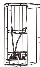
6 Run the cables so that they are not pinched between the chassis and back box.
