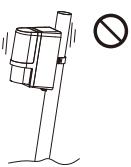
Do not install the unit in a location where trees, leaves, or other objects that may swing in the wind may block the beam.
