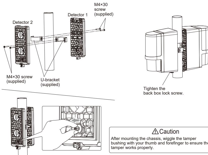
Tighten the back box lock screw.
